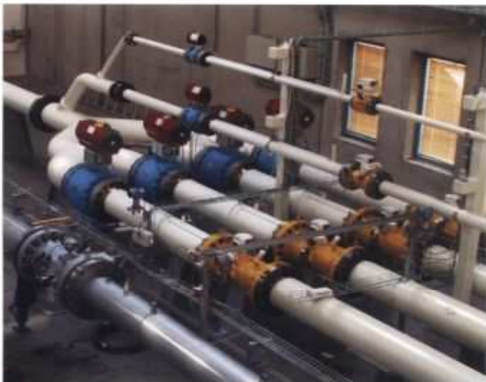
The national reference laboratory Force Technology in Vejen, Denmark. Calibration of gas flow meters.
