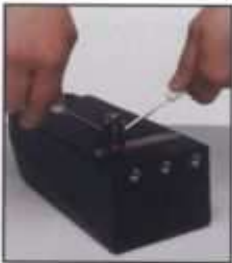
The spindle can easily be changed by using two screw drivers.
